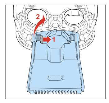
Remove the trimmer from the hairchamber by pushing the black nock by a small screwdriver inside the spring, to the inside.
